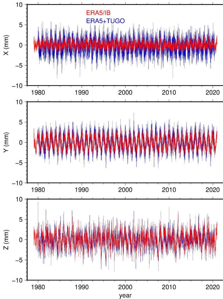
Figure 5: Geocenter motions due to atmospheric and induced ocean loading (ERA5/IB and ERA5/TUGO).
