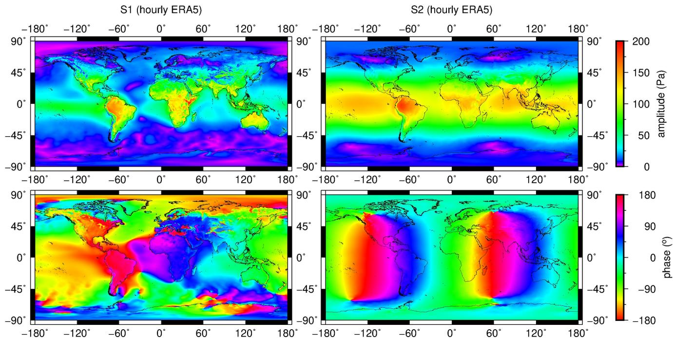
Figure 1: Amplitude (top) and phase (bottom) of S1 (left) and S2 (right) barometric tides computed from hourly ERA5 surface pressure (1980/01 - 2018/12).
