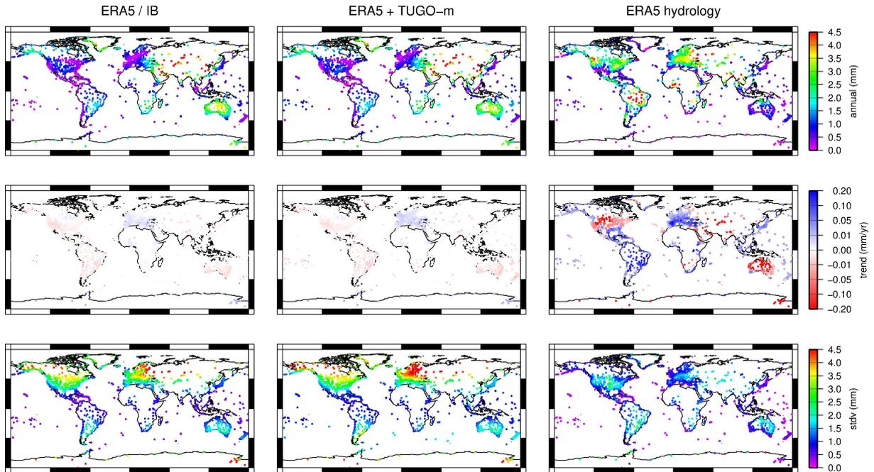
Figure 3: Annual amplitude (top in mm), linear trend (middle in mm/yr) and high-frequency variability (bottom in mm) of modeled vertical displacements at ITRF2020 sites (CF reference frame).
